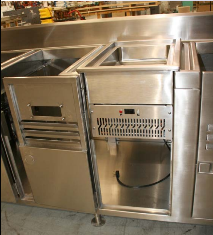
Illustration 2.C- Dual Serving Module Docked in Flex Serving Line Cabinet
