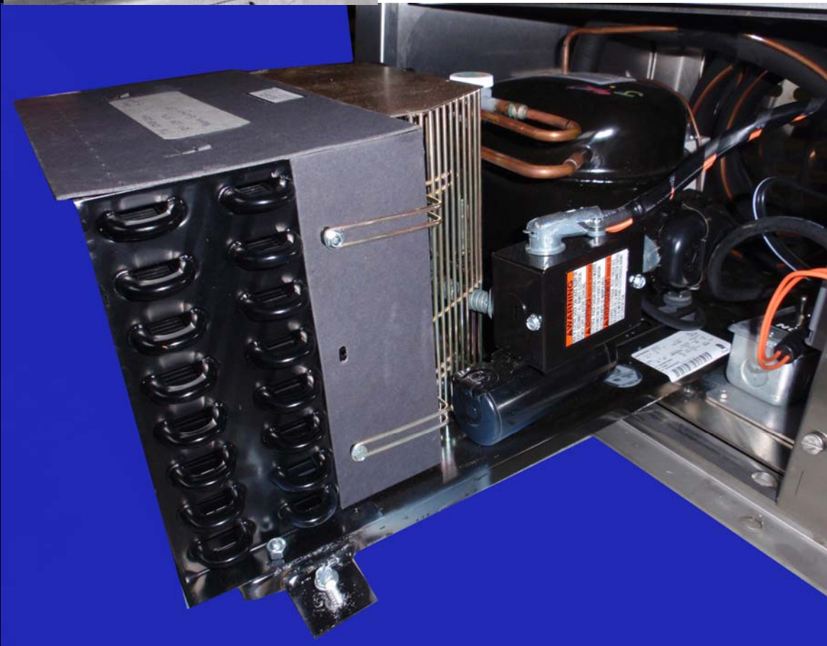
Illustration 2.B- Condensing Unit Assembly
