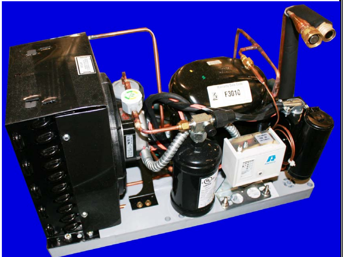
Illustration 2.B- Condensing Unit Assembly
