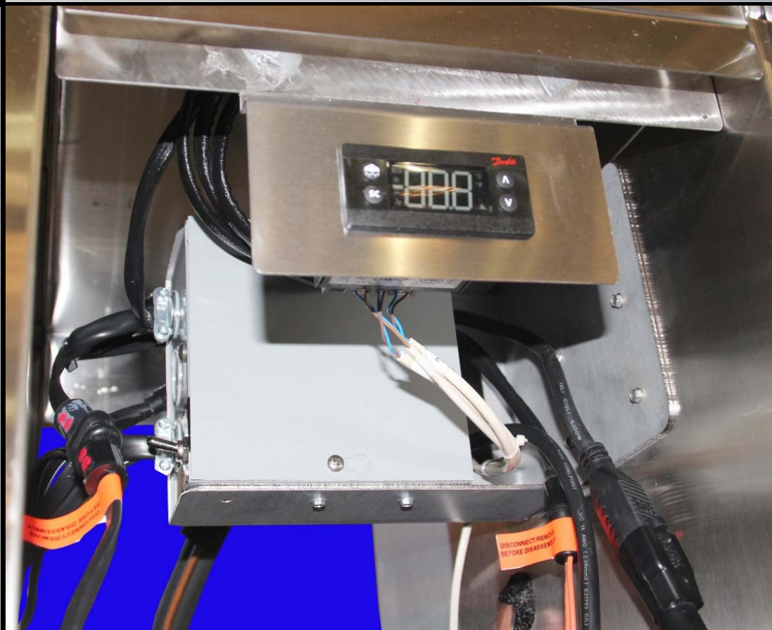
Illustration 2.A: Electronic Controller Assembly
