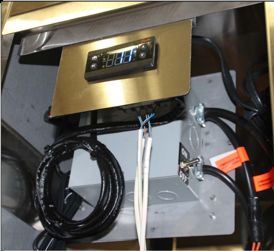
Illustration 2.A-RWTT65-PM Electronic Controller Assembly
